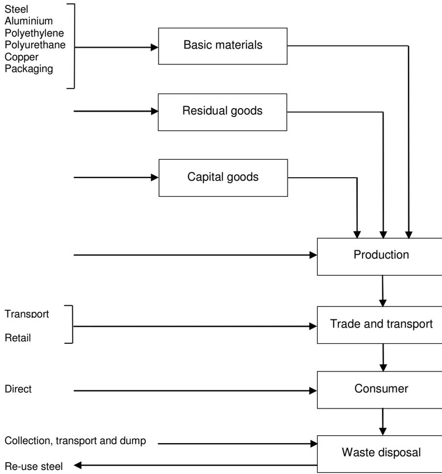
Figure #2. Flow chart of a refrigerator's life cycle.
