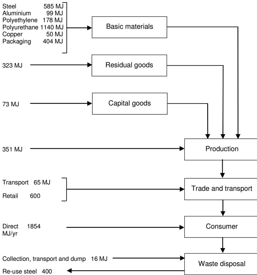
Figure #3. Flow chart of the life cycle of the refrigerator, together with the energy requirements in the various steps.
